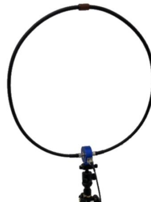
Picture 2: using corrugated coaxial cable to build a loop antenna
